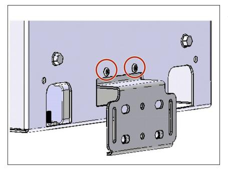
• Fix lower mounting bracket to the monitor's chassis with screws.
