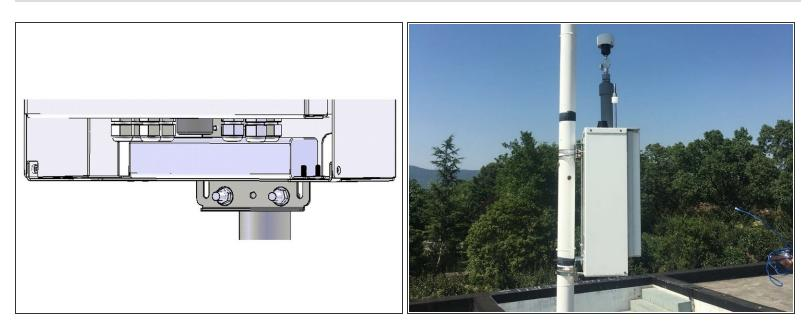
• Add nuts and washers and tighten the bottom U-bolt into position.
