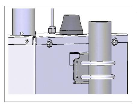
Align the slot on the back of the monitor with the top mounting bracket and lower the monitor on to the bracket.
