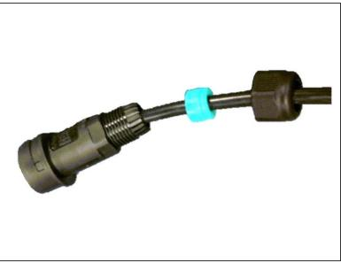
Thread the plug components over the power cable in the following order: nut gland, soft green gland, connector.
