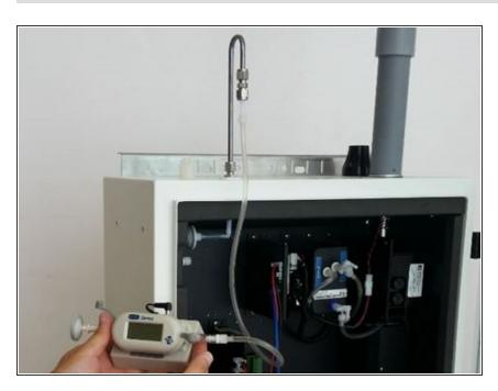
• <u>Perform a flow check</u> to make sure the inlet is fitted correctly and the sample pump is working properly.
