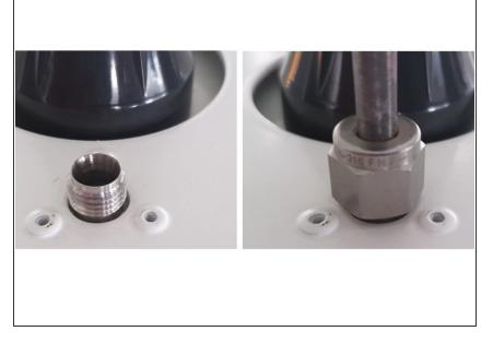
• Attach the inlet using a ¼ inch Swagelok compression fitting.
