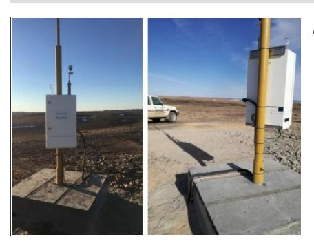
In this typical installation, a monitor is fixed to a pole that's set in a concrete pad.
