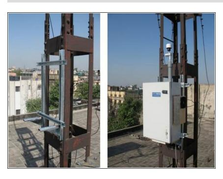
At this site, custom-made brackets secure the monitor to a strong radio mast.
