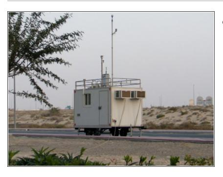
In this installation, the monitor is fixed to railing on the roof of a mobile trailer. A separate pole supports the wind sensor.
