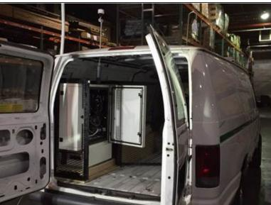
Alternatively, you can install a monitor in a van for mobile monitoring.
