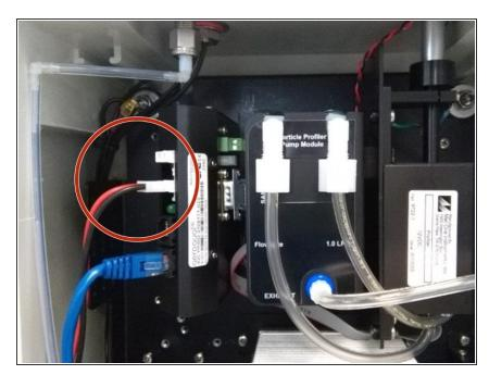
• Disconnect the sample pump from the monitor's electronics module.
