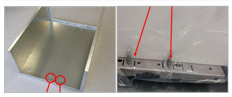
Carefully position the AQM 65 into the crate so the two supporting bolts at the end of the crate go through the AQM's mounting brackets.
