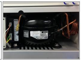
• Use a damp cloth to wipe the compressor tank and copper lines.
