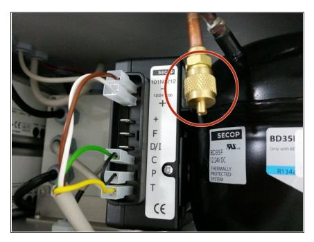
Unscrew the protective cap from the gas inlet, and put in a safe place because you will need to put it back on later.
