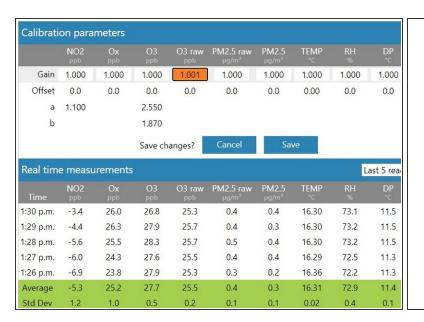
New offset = current offset + (gas reading / gain)
