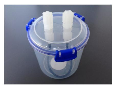
Fill the humidifier with water to the top of the label covering the black internal tubing.
