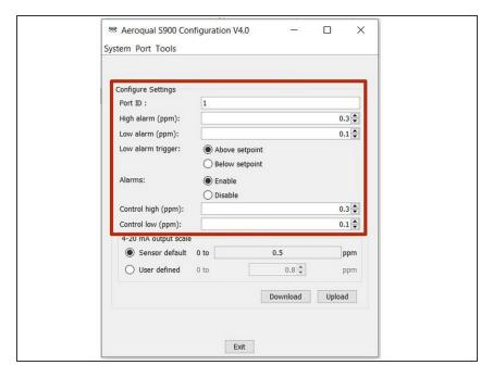
Configure your alarm or control output set points using Aeroqual's fixed monitor configuration software.
