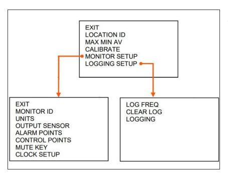
The Series 500 has a main menu and two sub menus from the MONITOR SETUP and LOGGING SETUP options.
