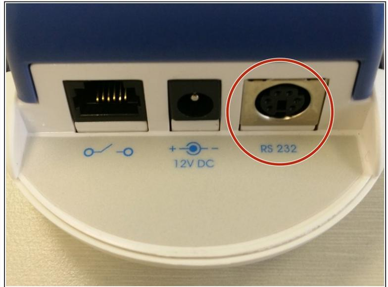
**⚠** Never attach the temperature and relative humidity sensor while the monitor is switched on as that can damage the monitor.
