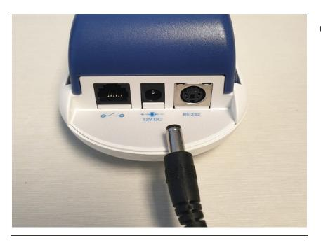
• Use the 12VDC AC/DC lithium smart charger to fully charge the battery.
