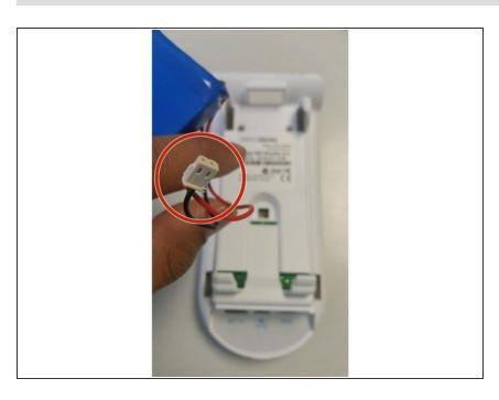
Insert the connector on the battery into the socket at the base of the monitor.
