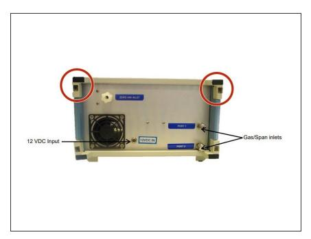
Unscrew the 2 top screws at the back of the AirCal 1000. The top plate should slide out easily.
