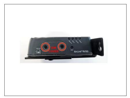
The SIM card slot is accessible on the left side of the device. Remove 2x screws and remove cover to expose the SIM card slots.
