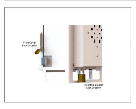
The AQY R can be locked to restrict access. A small padlock can be used to lock the front cover (maximum shackle diameter of 5mm), while another can be inserted in the back mounting tab to prevent the instrument from being removed from the wall mounting bracket. For further support, contact Technical Support.
