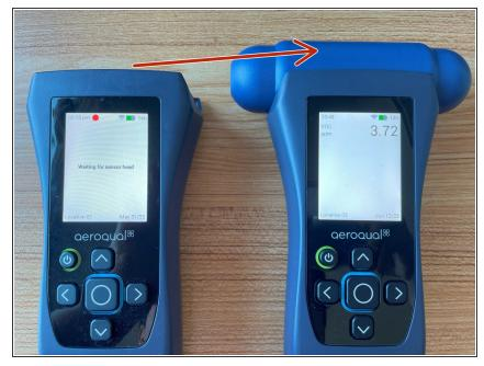
if you remove the gas sensor head from any Ranger base, and attach it to a different Ranger base, the Span will be retained
