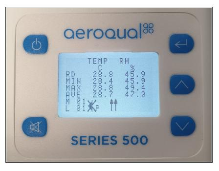
If a temperature / relative humidity sensor is fitted, its values alternate on screen with the measurement values from the sensor head.
