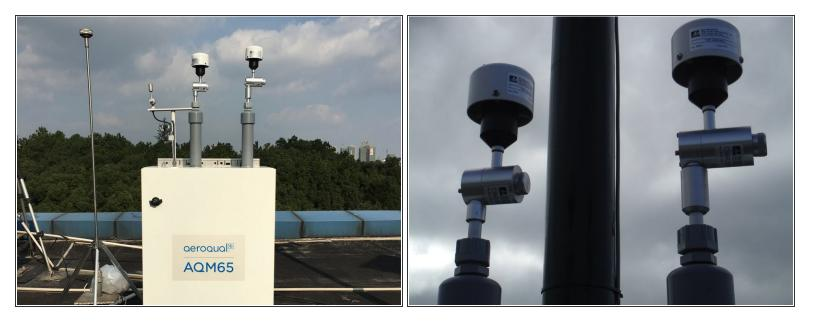
(i) If your AQM 65 has two particle monitors, the PM10 inlet is fitted on the right side and the PM2.5 is fitted on the left side.
