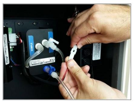
• Connect the inlet's heater plug to the plug coming from the optical engine.
