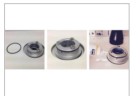
Attach an O-ring to the aluminum mounting ring on the roof of the monitor and apply a small amount of silicon lubricant.
