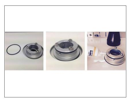
Attach an O-ring to the aluminum mounting ring on the roof of the monitor and apply a small amount of silicon lubricant.
