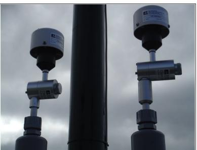
(i) If your AQM 65 has two particle monitors, the PM10 inlet is fitted on the right side and the PM2.5 is fitted on the left side.
