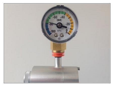
Fit the vacuum gauge to the inlet (above cyclone) and test for leaks (link).
