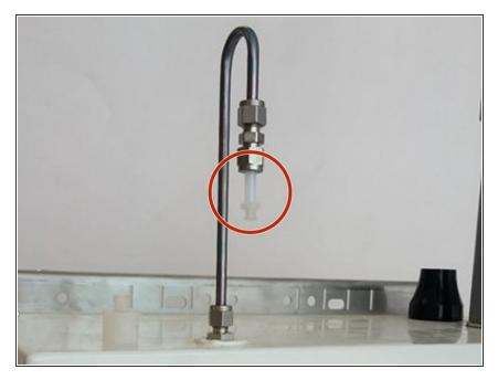
Attach the inlet flow adaptor.
