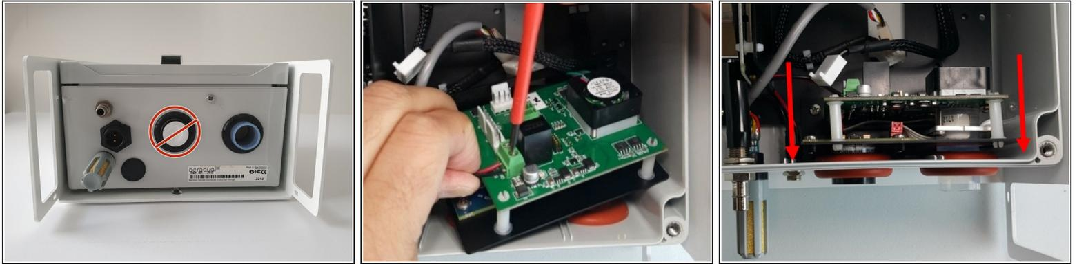
**⚠ Never directly touch the exposed NO<sub>2</sub> sensor at the bottom. If it becomes disconnected from your replacement sensor assembly, grip the sides of it when reconnecting.**
